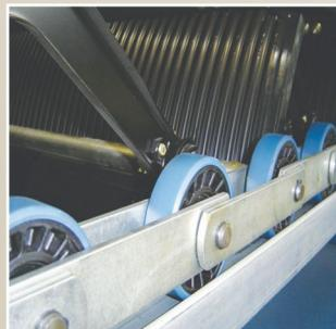
MakNet uses hydrolysis-resistant polyurethane step rollers. These are the most reliable rollers on the market. They ensure smooth running even in tropical and subtropical regions.
